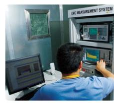
This is the Electromagnetic chamber where we test all products for compliance with standards such as FCC emissions, CE and safety. The facility represents a multi-million dollar investment and includes at least one machine that qoes "ping"
